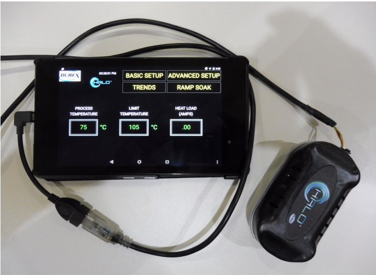
Modbus RTU Temperature Controller Monitoring
